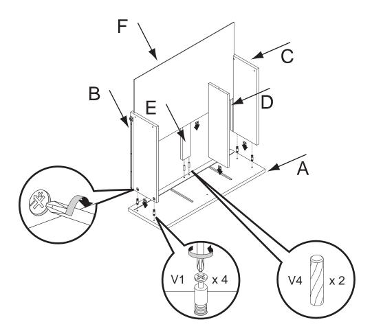
1. Attach board (B,C,D,E,F) to the front board (A) with cam screws (V1) and wooden dowels (V4). Turn the cam locks(on B&C) clockwise to secure.
